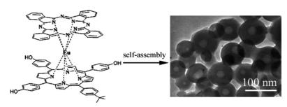
The sandwich-type mixed (phthalocyaninato)(porphyrinato)europium double-decker complex Eu(Pc)[T(OH)<sub>3</sub>PP] with three hydroxy groups at the *meso*-attached phenyl substituents of the porphyrin ligand as typical hydrophilic heads was designed, synthesized, and characterized. This amphiphilic double-decker compound formed hollow nanospheres during self-assembly.
