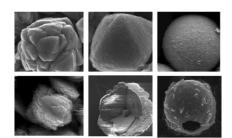
Nanoporous CuO microstructures with high surface areas and good CO catalytic activity have been synthesised by a facile carbonate-assisted hydrothermal route. The introduction of NaHCO3 plays an important role in the formation of the porous structure, while the molecular weight and concentration of poly(vinylpyrrolidone) (PVP) are critical in controlling product morphology.
