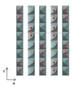
Four members of the new series  $\mathrm{NdMn}_{2-x}$   $\mathrm{Ru}_x\mathrm{O}_5$  (x=0.1, 0.2, 0.4, 0.5) have been investigated. The structures contain infinite chains of  $(\mathrm{Mn},\mathrm{Ru})^{4+}\mathrm{O}_6$  octahedra sharing edges. For x=0.5 the abrupt contraction of the c axis and the short (Mn,Ru)-(Mn,Ru) distances (2.60 Å) suggest the presence of Ru–Ru metal bonding within the chains.
