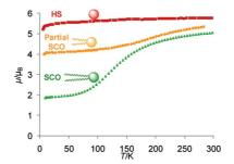
Thermal spin crossover (SCO) was induced in a high-spin  $Fe^{III}$  complex by alkylation of the ligand backbone. The SCO profile was responsive to chain length with partial crossover observed with  $C_6$  alkylation and full transition upon lengthening to  $C_{12}$ .
